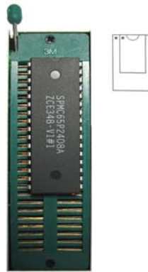
Figure 1-4 In-Circuit Programming fixture
