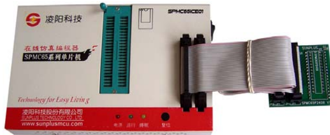
Figure 1-2 Extension Connectors to SPMC65X In-Circuit Emulator Adapter
